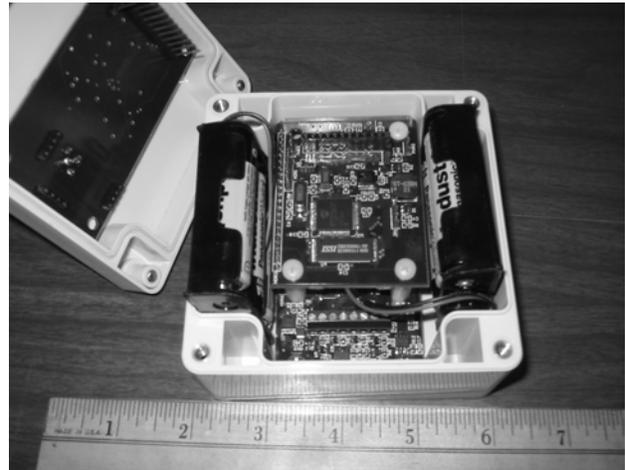
Figure 1. WiSARD hardware. The Brains board (center, between battery packs) controls and receives data from the Radio board (upper left, in box lid) and the Sensor Data (SD) board (bottom).
