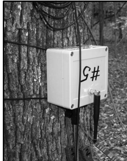
Figure 3. WiSARD sensor node deployed on tree trunk. Probe cables are connected at the bottom (behind the antenna).
