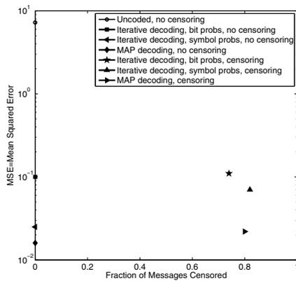
Figure 3. MSE vs fraction of messages censored for relay network.
