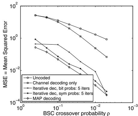
**Figure 1. MSE vs  $\rho$  for 3-node relay network without transmission censoring.**
