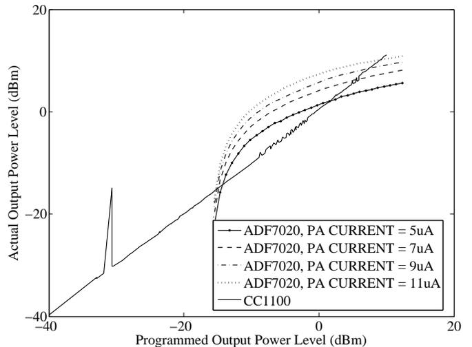
Fig. 5. Transmit power control accuracy for CC1100.
