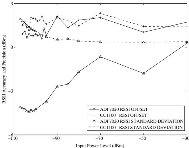
Fig. 4. RSSI accuracy and precision for the ADF and CC SIR's as a function of true received signal power.
