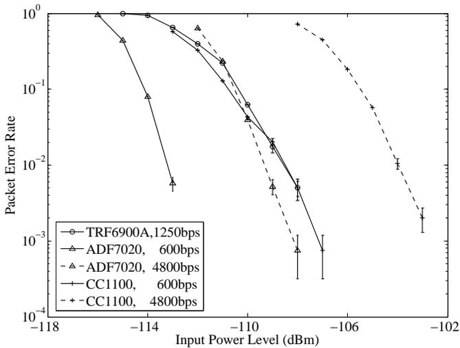
Fig. 1. PER as a function of received signal power for data rates of 600 bps (1250 bps for TRF) and 4800 bps.
