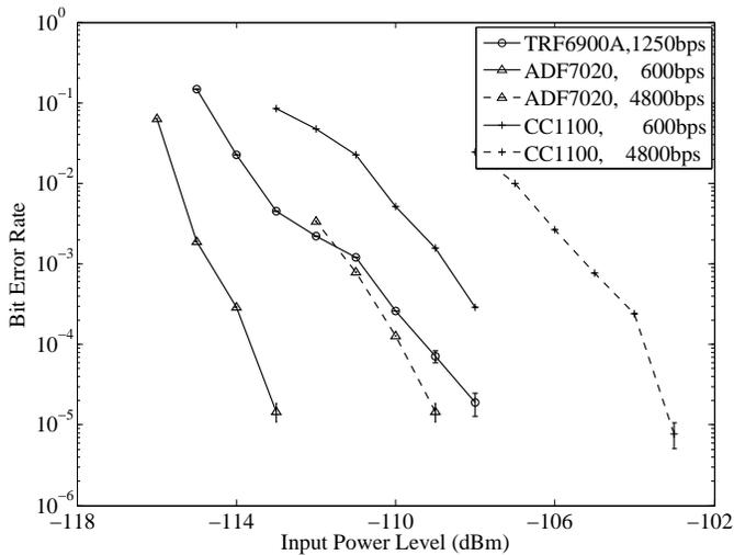
Fig. 2. BER as a function of received signal power for data rates of 600 bps (1250 bps for TRF) and 4800 bps.
