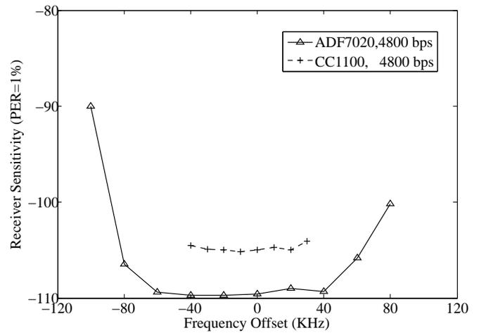
Fig. 3. Receiver sensitivity (at 1% PER) as a function of Tx-Rx frequency offset.
