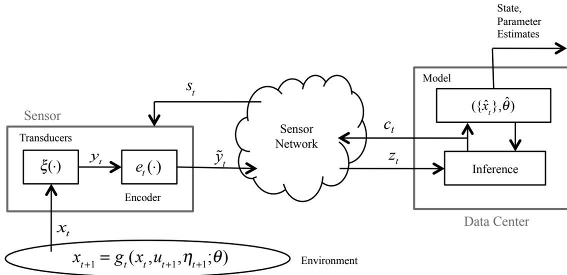
Fig. 1. Block diagram of asymmetric data processing. Processes  $x_t$  that capture the state of the environment or its covariates are transduced, encoded using simple algorithms, and sent to a data center, accumulating uncertainty at each step. Model-based inference is performed on the received data that is a corrupted version of the encoded vector data stream  $\tilde{y}_t$ . Adaptation of compression and transmission censoring is steered via commands  $c_t$ .
