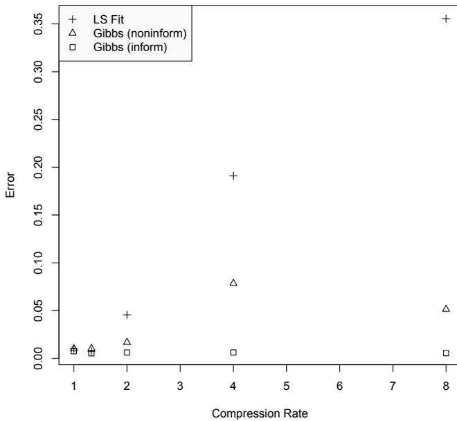
Fig. 2. Fractional error for estimation of model parameter  $b_0$  for least-squares fit and Gibbs samplers with non-informative and informative priors. Higher compression rate means less data sent and correspondingly less energy used.
