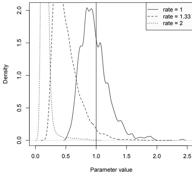
Fig. 3. Posterior density estimates (smoothed with Gaussian kernel) of process noise variance  $\sigma_x^2$  for different compression rates show convergence as rate decreases. (The true variance value of 1 is shown.)
