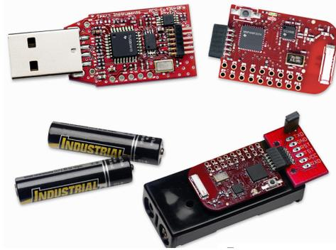
Fig. 1. Texas Instruments eZ430-RF2500 development tool. USB programmer/communication interface is at upper left. Two 2.4 GHz wireless MCU nodes are at right; one node (lower right) has an attached battery carrier.
