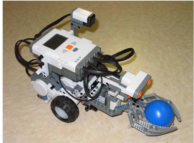
**Figure 5: A picture of the basic ARCHIE MINDSTORMS robot: a three-wheeled design with a grasping arm and a number of mounted sensors along with the NXT processor brick.**
