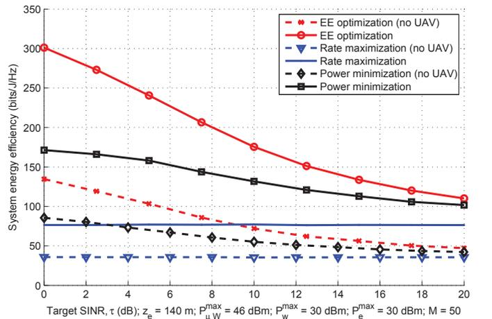
Fig. 5: System EE versus target SINR  $\tau$ , both with and without the UAV tier.
