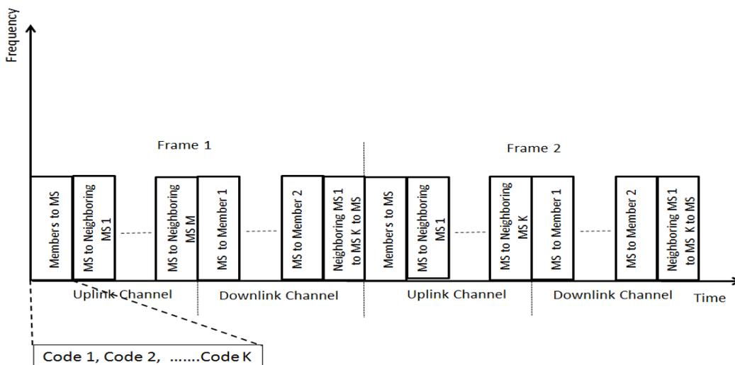
Figure 5. The frame structure of hybrid TDMA/CDMA system (CDMA Centric)
