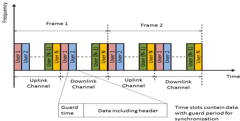
Figure 1. TDMA/TDD Frame structure
