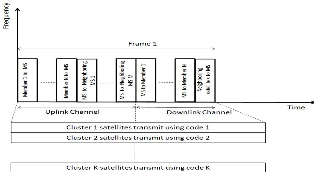
Figure 4. The frame structure of hybrid TDMA/CDMA system (TDMA Centric)
