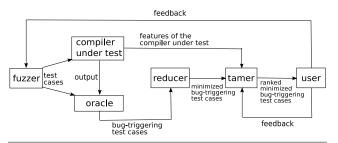
Figure 2. Workflow for a fuzzer tamer
