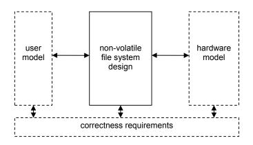
Fig. 1. Sandwich Model for File System Verification
