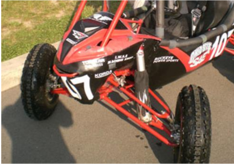
Figure 5 Double A-Arm Suspension Geometry, Fabricated from Round Tubing
