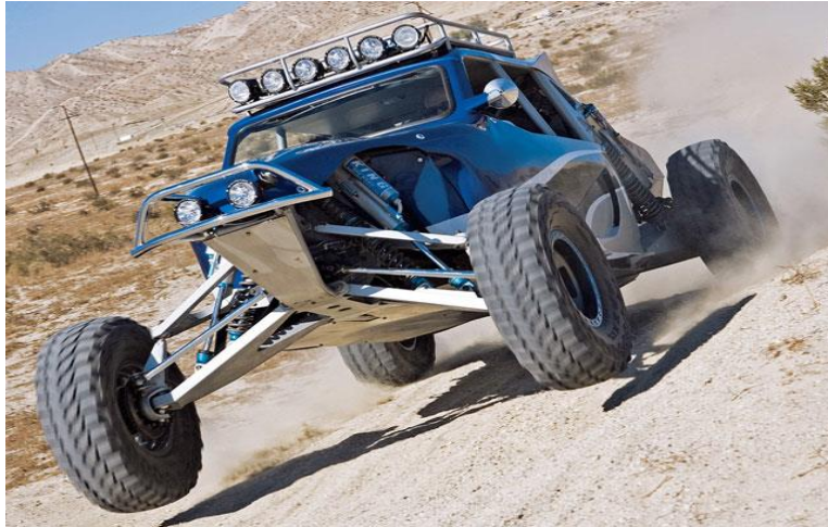
Figure 6 Double A-Arm Suspension Geometry, Boxed-Style Fabrication
