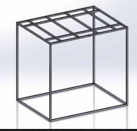
Figure 19. CAD of Fully Assembled Room Frame
