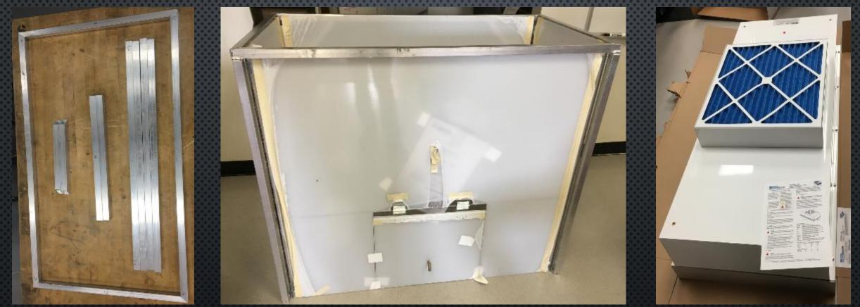
Figure 9. Cut Aluminum Frame
