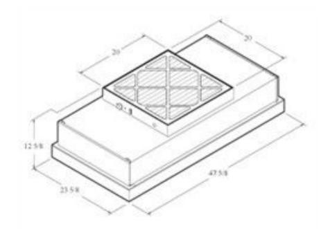
Figure 2: 2X4 Fan Filter Unit [3]
