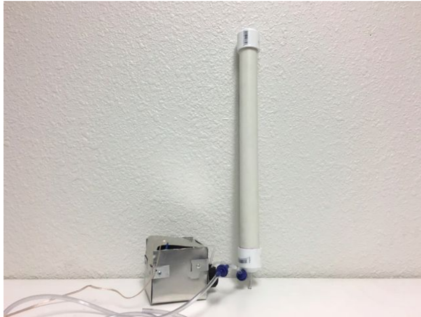
Figure 4 - The Pump Assembly
