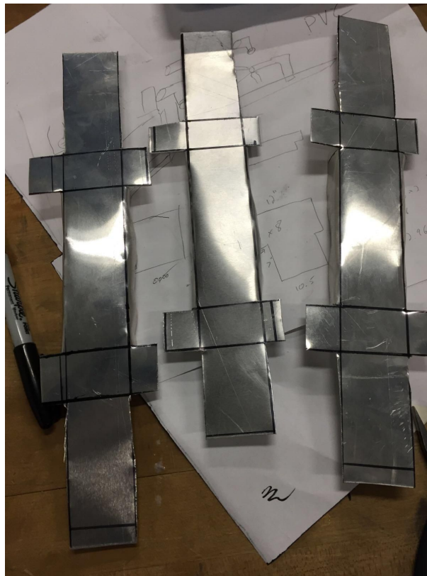
Figure 8 - Templates of Inserts in Air Chambers
