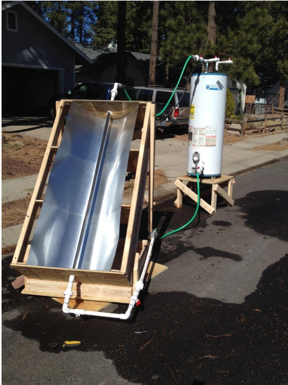
Figure 1: Parabolic Collector Design
