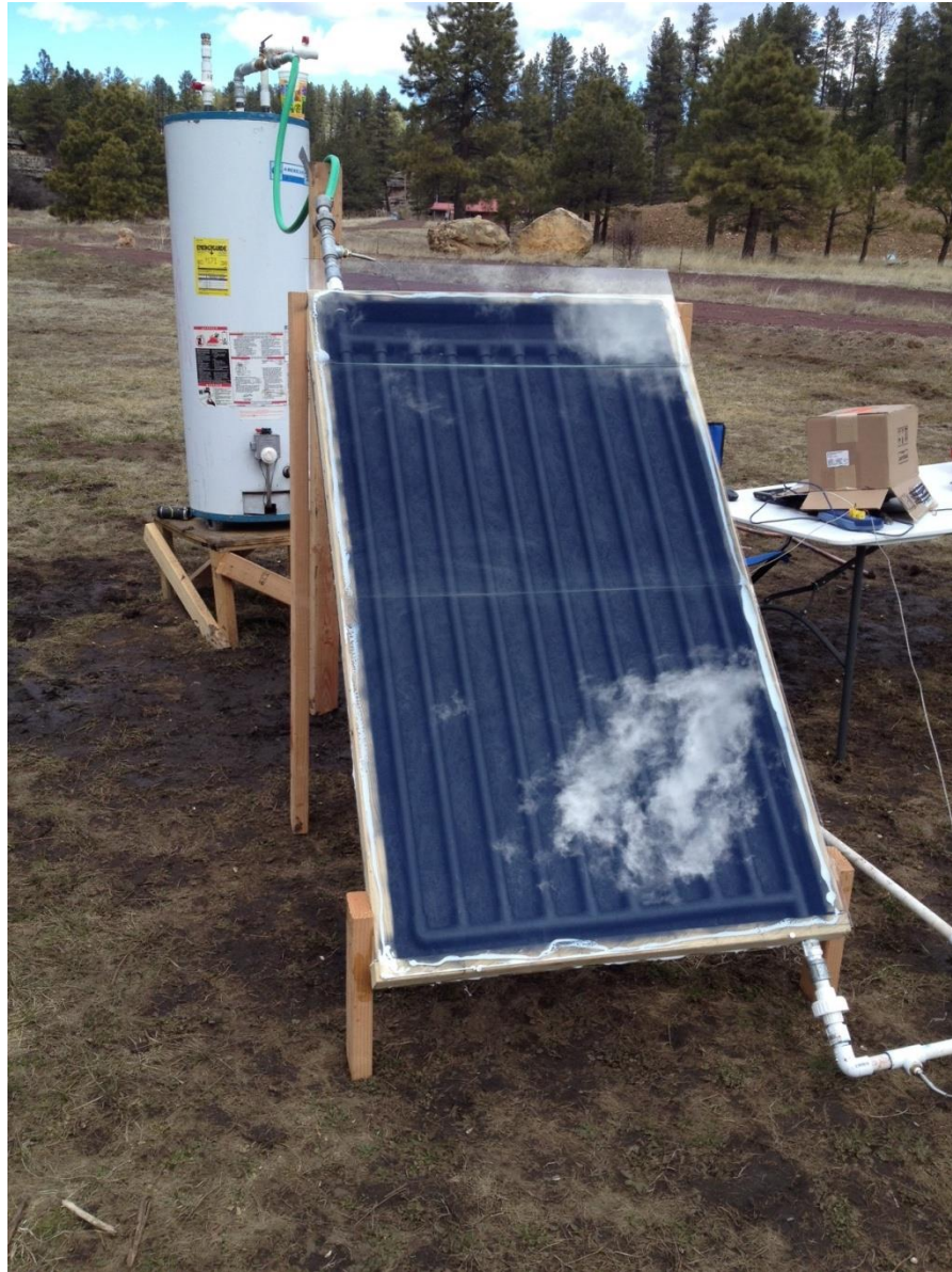
Figure 2: Flat plate collector design
