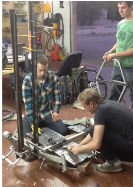
Figure 5.12- Frame Realignment Set Up
