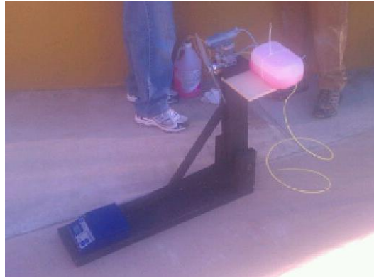
Figure 3: Static thrust test stand
