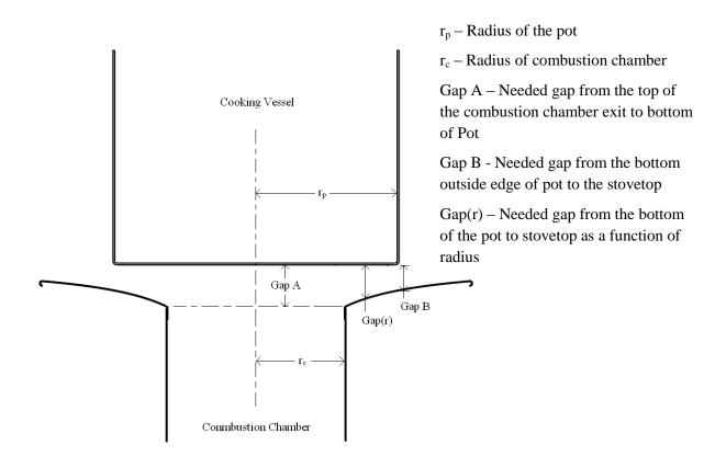
Figure 9 - Schematic of Stove and Flat-bottom CookingVessel
