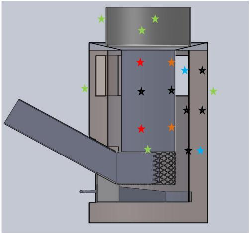
Figure 18 - Cross-sectional view of stove with placement of the thermocouples
