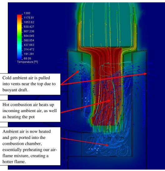
Figure 7 - Design 3 Flow Simulation, Temperature Profiles
