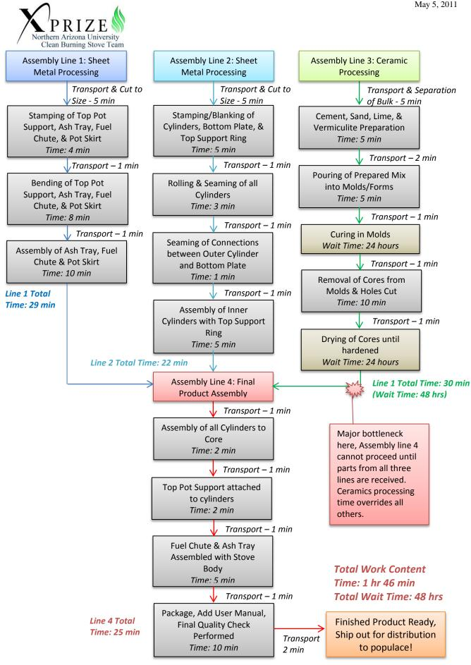
Figure 26: Proposed Workflow for Manufacturing
