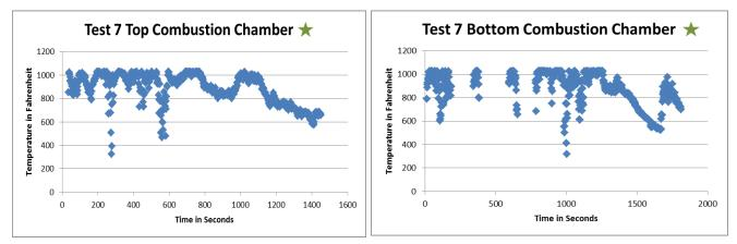
Figure 23: Top of Combustion Chamber Temperature-Time Response
