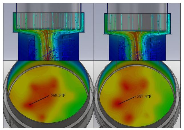
Figure 11 - Comparison of Cone-Shaped Stovetop and Ideal Stovetop Shape for a Flat Bottom Cooking Vessel
