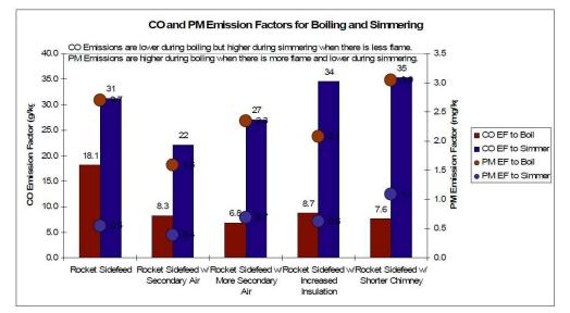
Figure 25 – CO and PM Emission Factors for Boiling and Simmering from Aprovecho Research Center
