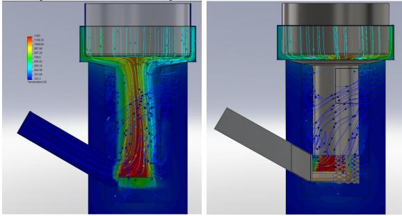
Figure 15 – Cross-section of Prototype 2 Model 1 - Temperature Plot (293-1300K)
