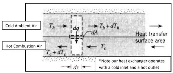
Figure 8 - Schematic of a Cross-Flow Heat Exchanger, Section view of one "wall" only, does not show the inlet and outlet ports.
