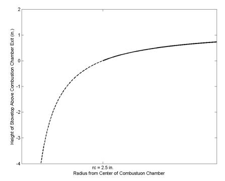
Figure 10 - Ideal Stovetop Shape as a Function of Radius for a 2.5 in. Radius Combustion Chamber (Solid line is where the actual stove geometry starts, i.e. the radius of the combustion chamber)
