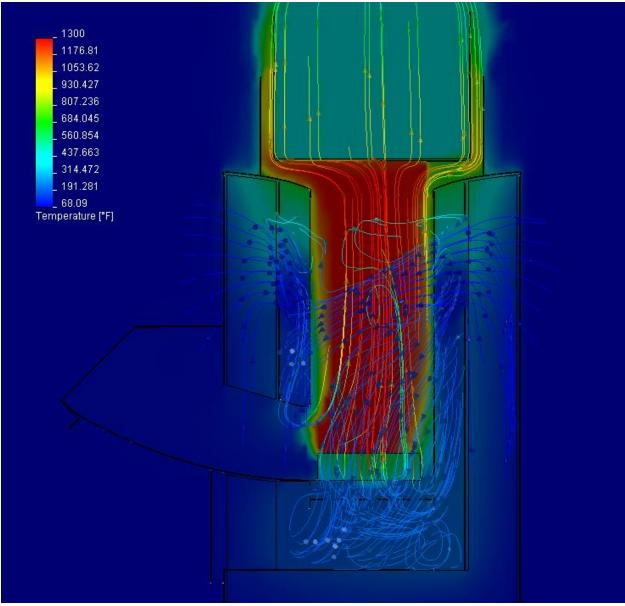
Figure 17 - Cross-section of Prototype 3 Theoretical Model Temperature Plot
