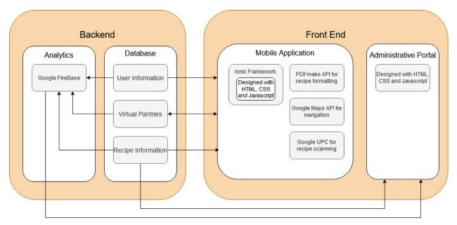
The system diagram for the application and supporting technologies.
