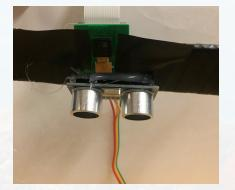
Figure 1: Ultrasonic Ranging Module on Prototype. Photo by Hashem Albhrani.
