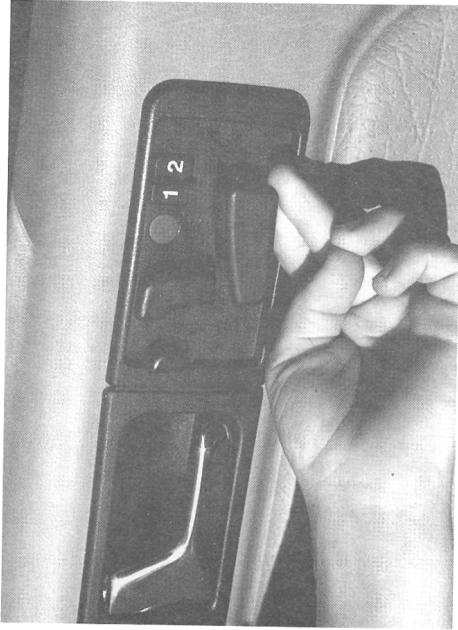
1.13 Seat Adjustment Control from a Mercedes-Benz Automobile. This is an excellent example of natural mapping. The control is in the shape of the seat itself: the mapping is straightforward. To move the front edge of the seat higher, lift up on the front part of the button. To make the seat back recline, move the button back. Mercedes-Benz automobiles are obviously not everyday things for most people, but the principle doesn't require great expense or wealth. The same principle could be applied to much more common objects.
