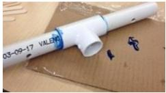
Figure 9. PVC adhesive on T-Shaped Section
