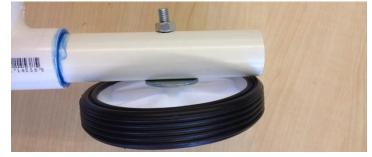
Figure 10. Wheel Washer Placement
