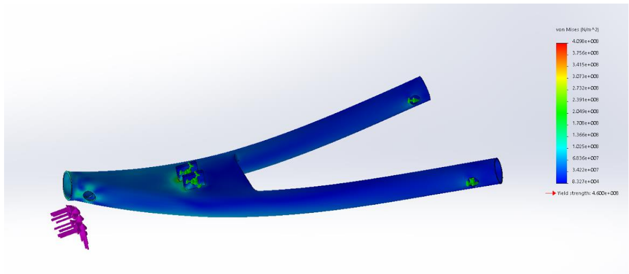
Figure 9: Vertical impact final FEA stress printout
