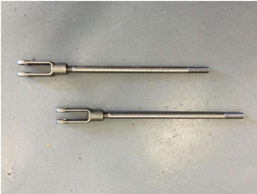
Figure 21: Manufactured Tie Rods with Clevis Joints
