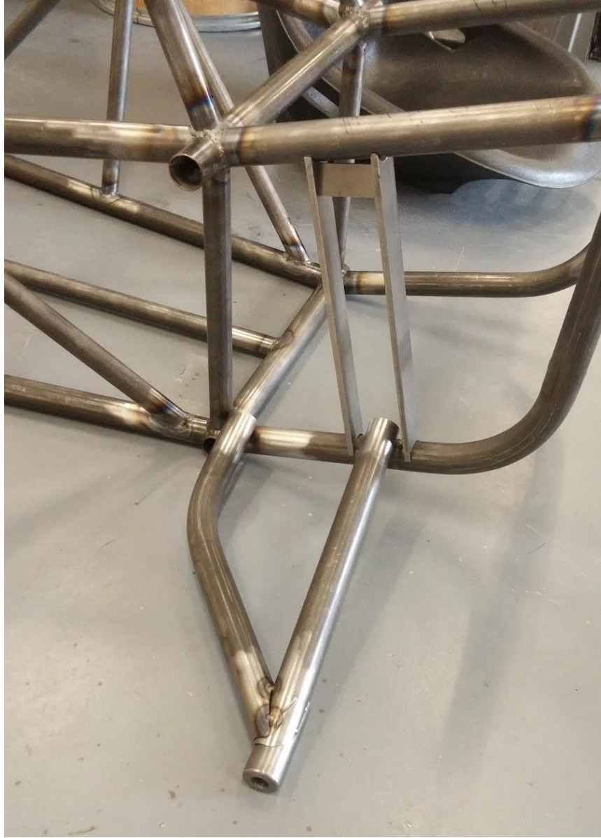
Figure 4 Mockup of lower A-arm and mounting tab
