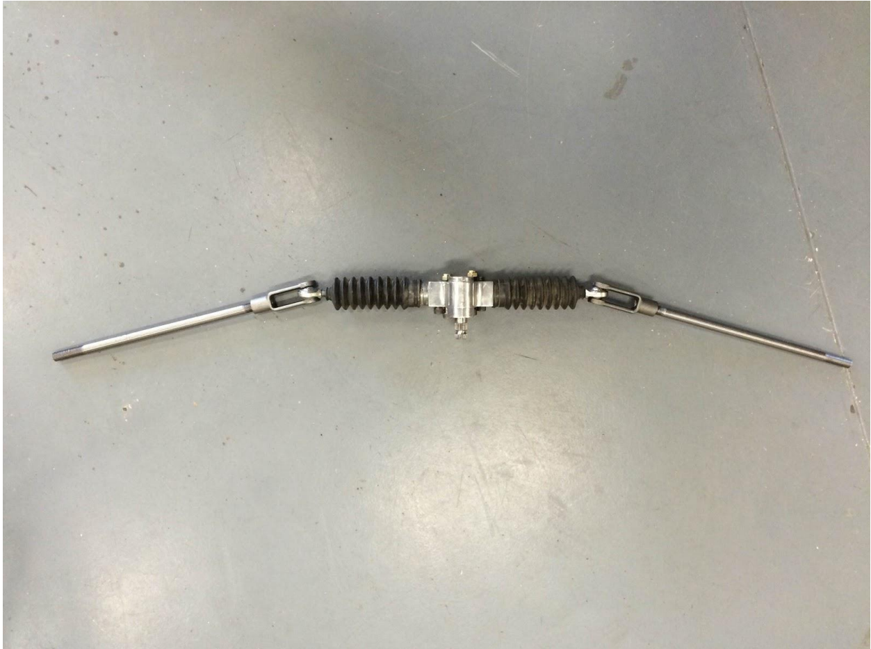
Figure 22: Rack and Pinion attached to manufactured Tie Rods
