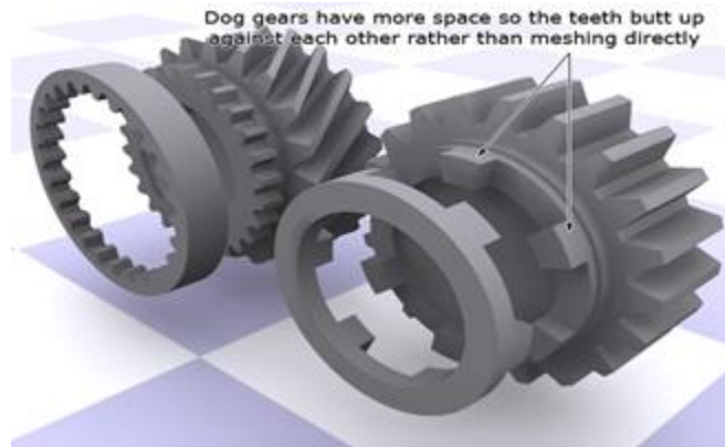
(Figure 2.1, Manual (left) Vs. Sequential (right) dog ring)
