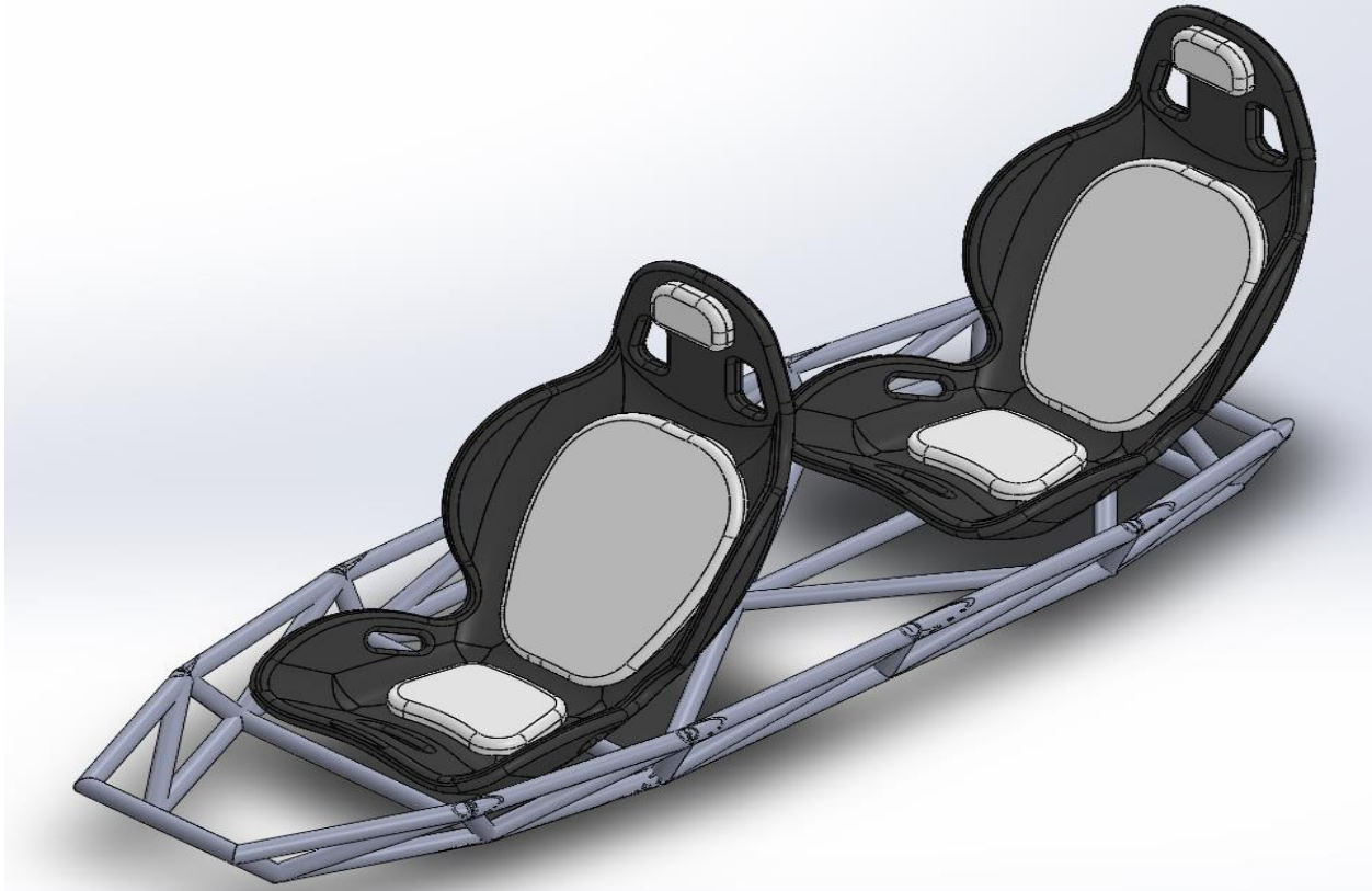
Figure 18: The go-kart frame that utilizes a wide spacing to allow for storage and low ride
