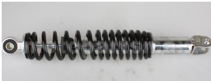
Figure 38: 13.8” Rear Shock Absorber
