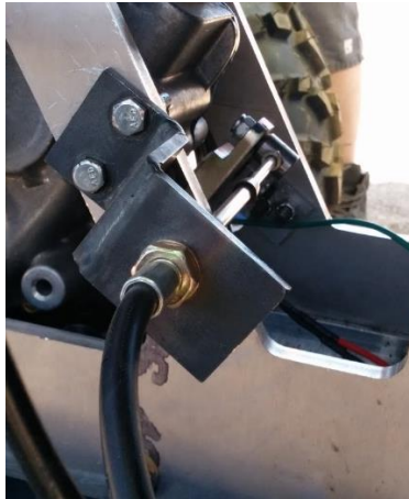
Figure 16: Assembled Shifting Cable Lock and Shifting Lever
