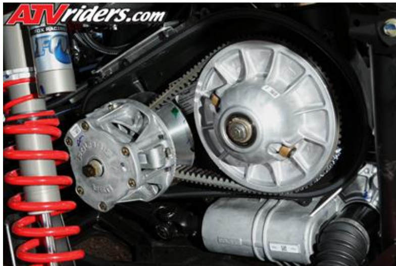
Figure 3: Rubber V-belt CVT (Source: atvriders.com)
