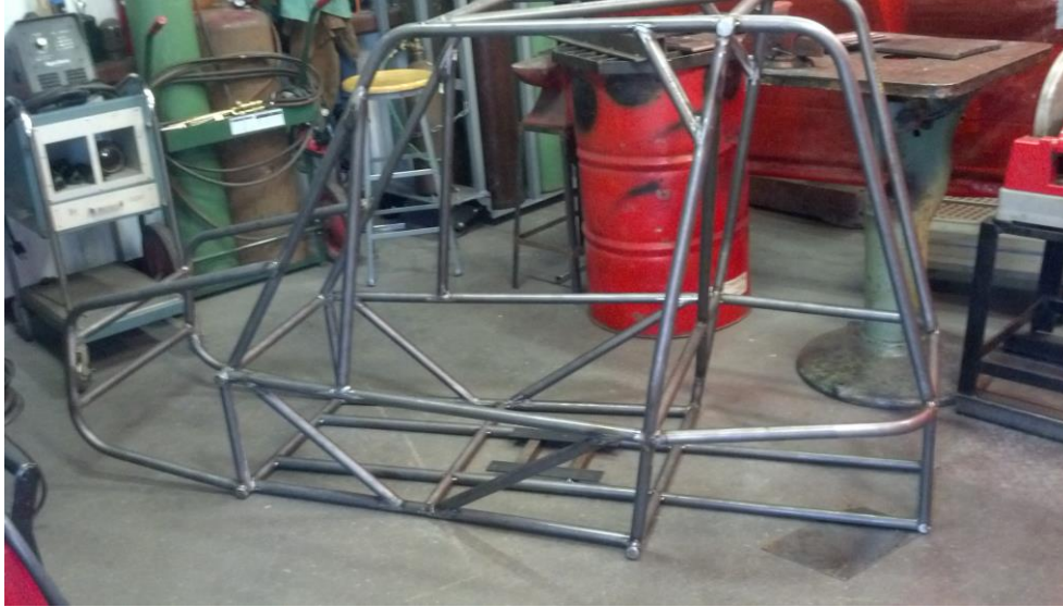
Figure 3. Current state of the frame with the rear end and seat mount installed.
