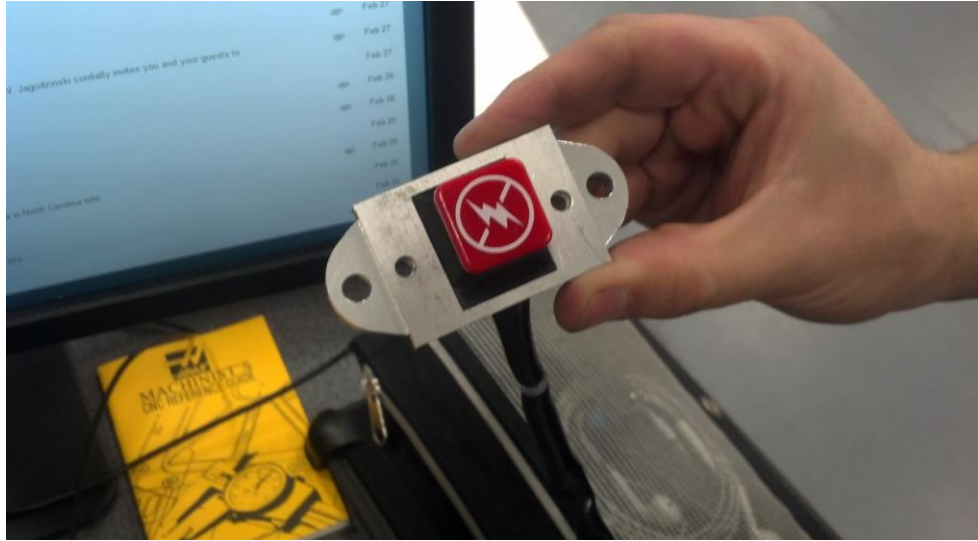
Figure 6. Finished mount with switch installed.
