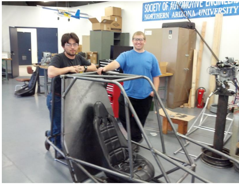
Figure 4. Dry-fit of the firewall.
