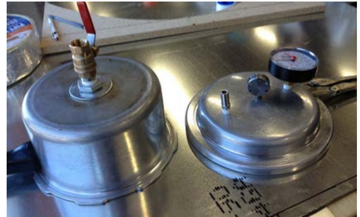
Figure 14: Modified Pressure Vessel
