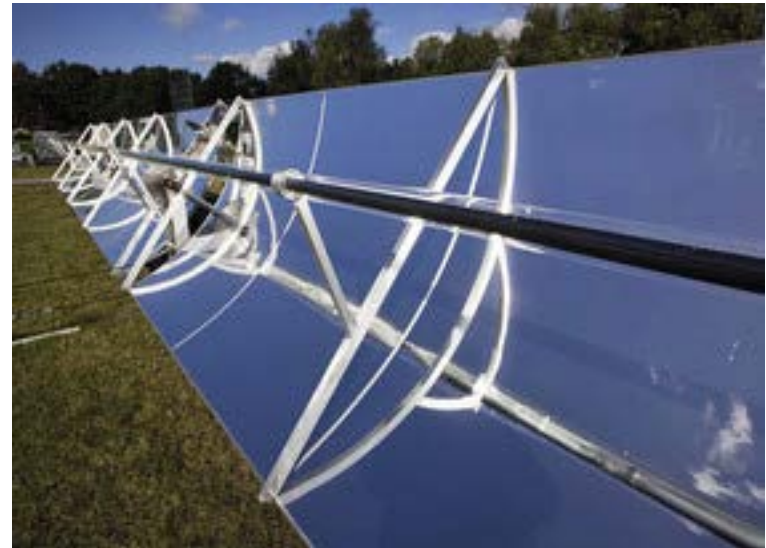
Figure 19: Solar Parabolic Trough
