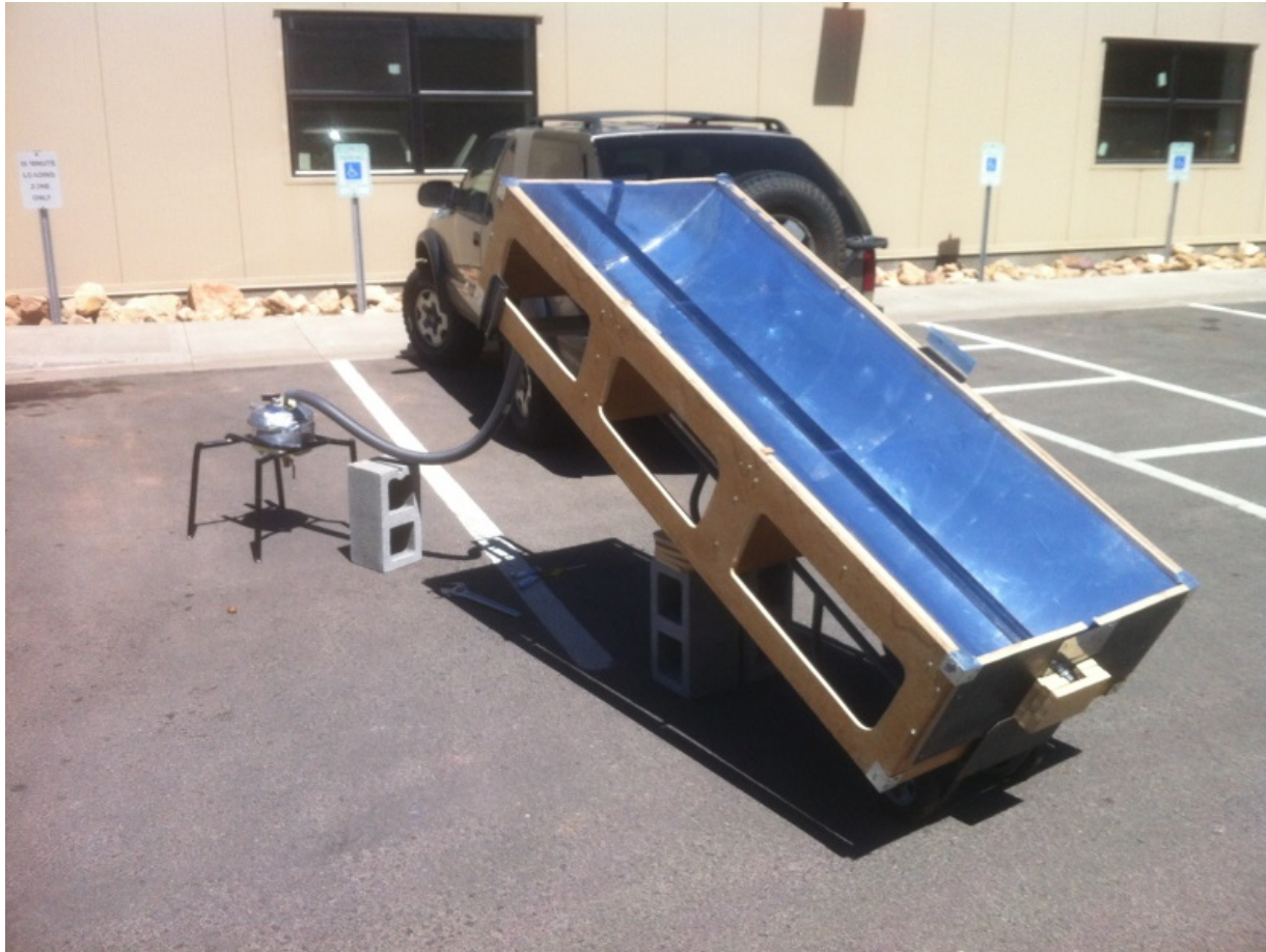
Figure 8: Solar Autoclave Final Design
