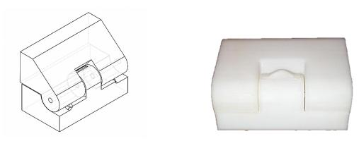
Figure 3 - Hinge prototype
