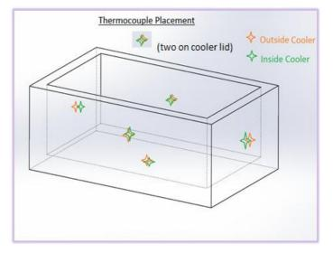
Figure 2: Thermocouple placement
