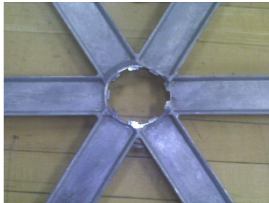
Figure 13: Spline fabricated into rear wheel sheave
