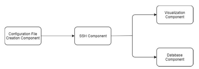
At a high-level, the architecture consists of four basic components:
