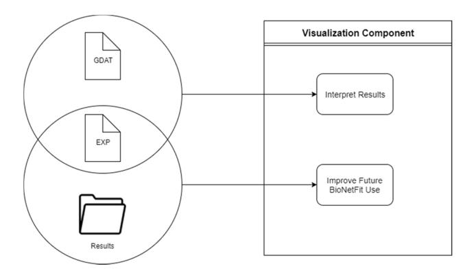
In general, visualizations that help interpret results will use individual GDAT files (which show the values of observables over time in a generation) and EXP files. Visualizations that help the user improve their usage of BioNetFit will use the entirety of the results folder, looking at GDAT files from every simulation in every generation. Some visualizations may be useful for both interpreting the results and improving BioNetFit usage.
