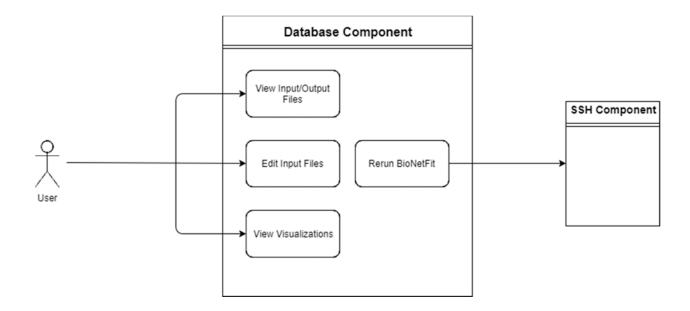
The Database component will allow the user to view input files (BNGL, EXP, configuration file), output files (best-fit GDAT files and generational GDAT files), and visualizations. It will also allow the user to quickly edit any of the input files and rerun BioNetFit on Monsoon using these new files.
